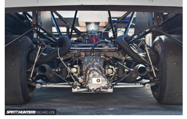
A peek under the rear, through the massive opening where the rear panel normally would be, answers these questions. Graeme's Charger, for all intents and purposes, is draped across a Lola T190 Formula 5000 open-wheeler. Taking pride of place in the rear is a Hewland transaxle, located by a custom cradle which utilises the Lola suspension components and uprights. Up front it's remarkably similar, the tube-frame chassis making use of the Lola uprights and suspension pick-ups.
